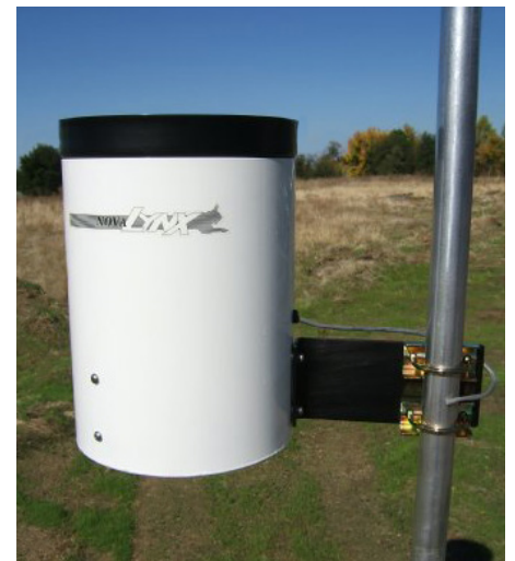
(Illustration - "tipping bucket" rain gauge)
