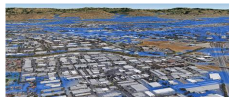
Three-dimensional extent for a 100-year flood for San Jose, California. (Source: IF)
